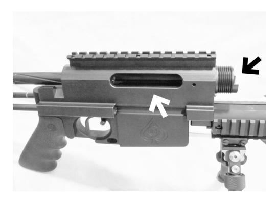
• General cleaning of the receiver consists of dusting off the outside of the receiver, cleaning the barrel threads with a toothbrush and wiping out the bolt pathway with a toothbrush or piece of rag. Recoat the inside of the receiver with a light coat of oil/CLP. To clean the trigger remove the pistol grip and magazine guide plate. This exposes the bottom of the trigger group itself.
